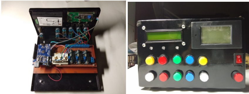
Figure 4. The PWM Value Control System and RGB (Red, Green and Blue) Lamp
